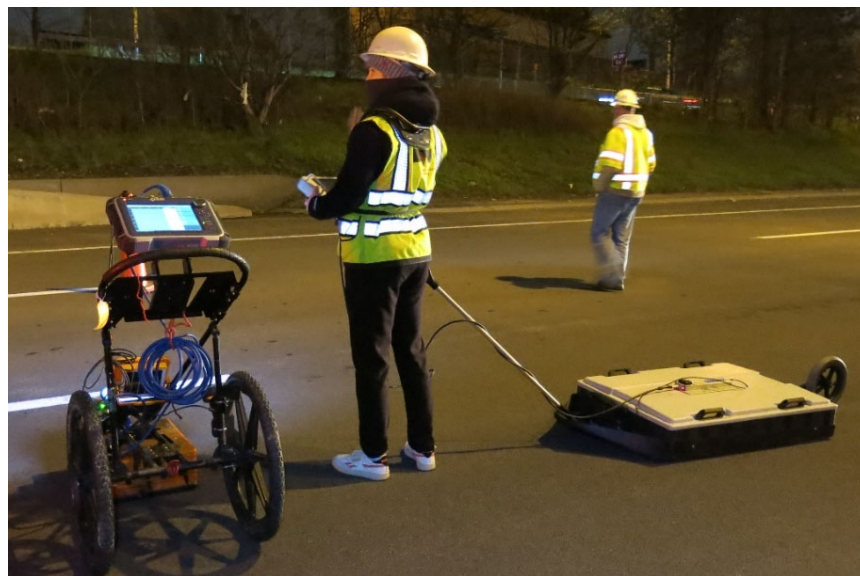
Figure 2. Picture of the GPR systems used during the field work. (Left) the 270 MHz GSSI GPR pushcart system and (right) the pulled 80 MHz Mala system.
